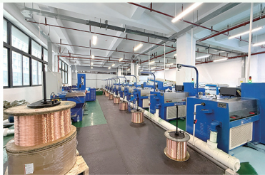
Inhouse Copper Wire Production
